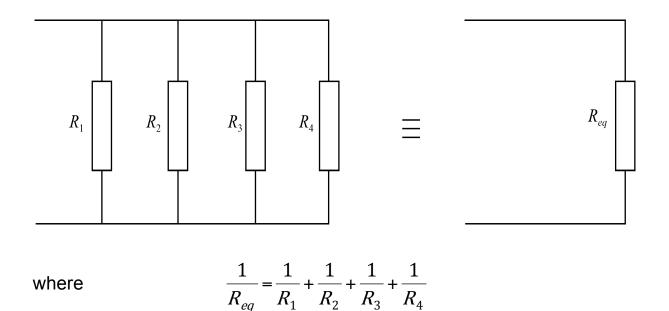
Since the inverse of resistances is involved in this case it is sometimes more convenient to work in terms of conductances, G(= 1/R). In this case if there are *N* such elements of conductance  $G_n$
