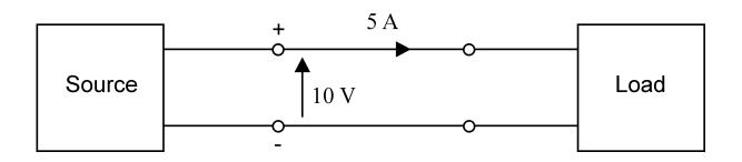
Here a power 5 A x 10 V = 50 W is transferred from the source to the load.
