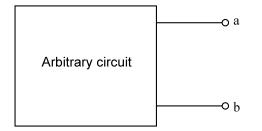
Consider an arbitrarily complicated **linear** circuit in which we only have access to two nodes, a and b. We can measure the voltage  $V_{ab}$  and extract a current  $I_a = -I_b$ . If the circuit is linear, there must be a **linear** relation between this voltage and current and a graph of voltage *vs.* current will be a straight line:
