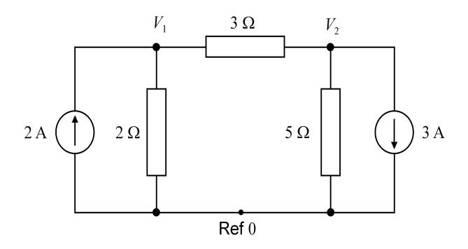
We begin by introducing node voltage  $V_1$  and  $V_2$  with respect to the reference node 0. In general if a circuit has *n* principal nodes we need (*n*-1) simultaneous equations to solve the circuit.
