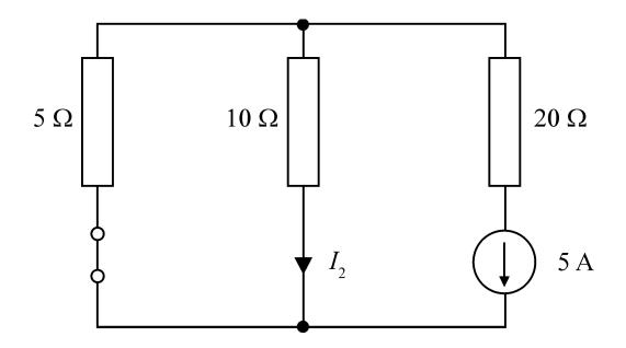
The 5A current is now split between  $5\Omega$  and  $10\Omega$  resistors in parallel. The same voltage is developed across both resistors thus
