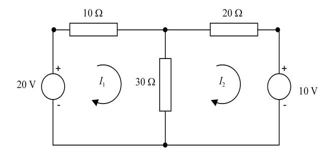
We use this notation to indicate that a current  $I_1$  flows through the 10 $\Omega$  resistor and a current  $I_2$  through the 20 $\Omega$  resistor. The current through the 30 $\Omega$  resistor, on the other hand, is given by  $I_1$ - $I_2$  "downwards" or  $I_2$ - $I_1$  "upwards".
