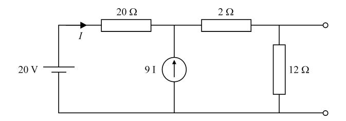
We begin by calculating the open circuit voltage and note that, since a current of 9I + I = 10I flows through both the 2 $\Omega$  and 12 $\Omega$ resistor under these conditions that  $V_{oc} = 12 \cdot 10I = 120I$ . We may find I by writing a KVL equation around the outer perimeter as
