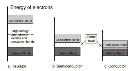
The Fermi level is the top energy level that would be occupied at absolute zero. At higher temperatures, the electrons are excited to higher energy levels.
