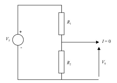
The current flowing through the two resistors is  $V_s/(R_1 + R_2)$  and hence the voltage appearing across the resistor  $R_2$  is given by
