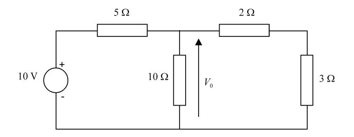
We first note that the  $2\Omega$  and  $3\Omega$  resistors are connected in series and so may be replaced by a single  $5\Omega$  resistor. Thus the circuit can be redrawn as on the left below:
