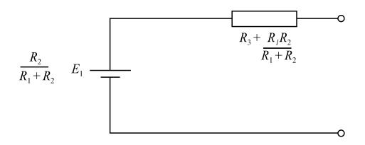
At this point another possibility may occur to you. Suppose we set the sources to zero in our arbitrary circuit (as we did with superposition earlier). In this case it is a simple matter of setting  $E_1$ to zero. The circuit is now entirely resistive and the resistance between the terminals is just  $R_3$  in series with a parallel combination of  $R_1$  and  $R_2$  giving us the above Thévenin resistance more directly. Now try another example:
