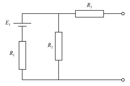
$E_1$  in series with  $R_1$  comprise a Thévenin circuit and can be replaced by the Norton circuit of  $I_N = E_1/R_1$  in parallel with  $R_1$ .
