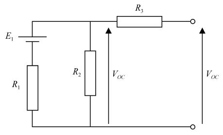
Since current flows only in the left hand loop  $(=E_1/[R_1 + R_2])$  it is simple to write
