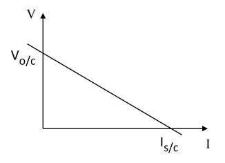
The intercept with the voltage axis occurs when *I* is zero and can be measured as the **open-circuit voltage**,  $V_{o/c}$ . The intercept with the current axis occurs when *V* is zero and can be measured as the **short-circuit current**,  $I_{s/c}$ . We can therefore represent it by the equation:
