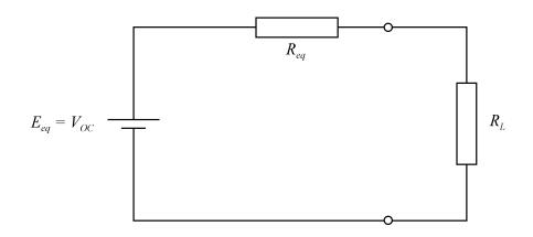
The current flowing in the circuit  $I = V_{oc} / (R_{eq} + R_L)$  and the power dissipated in the load, P, is given by
