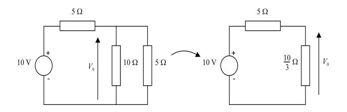
However the 10 $\Omega$  and 5 $\Omega$  resistors are now seen to be connected in parallel with the desired voltage  $V_0$  appearing across both of them. This combination may be replaced by a single resistor of value  $\frac{10.5}{10+5} = 10/3\Omega$  as shown in the right hand diagram. This may, if necessary, be further re-drawn in the standard voltage divider configuration as
