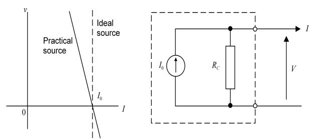
Since the current through the resistor  $R_c$ , is  $I_0 - I$  'downwards', the terminal voltage is given, by Ohm's law, as  $V = (I_0 - I)R_c$ . Therefore we may write
