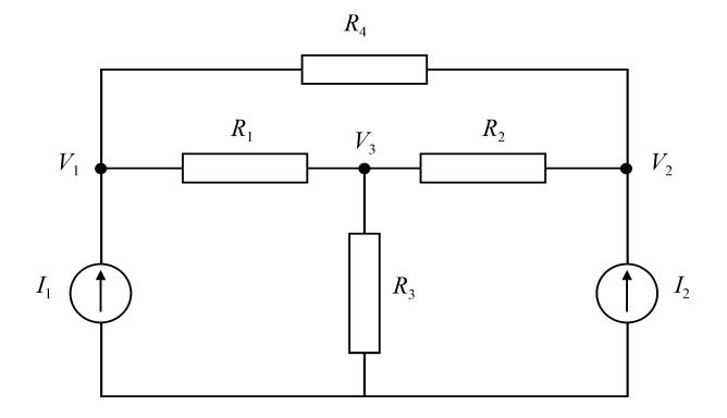
where we have introduced node voltages,  $V_1$ ,  $V_2$  and  $V_3$ . The node-voltage equations may be written as
