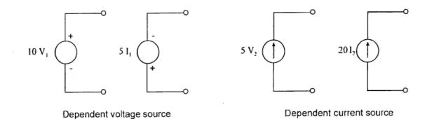
where  $V_1$ ,  $I_1$ ,  $V_2 \& I_2$ , are voltages and currents somewhere else in the circuit. Although the dependent source concept may seem a little farfetched at the moment, we will have cause to return to it in connection with transformers and transistors.
