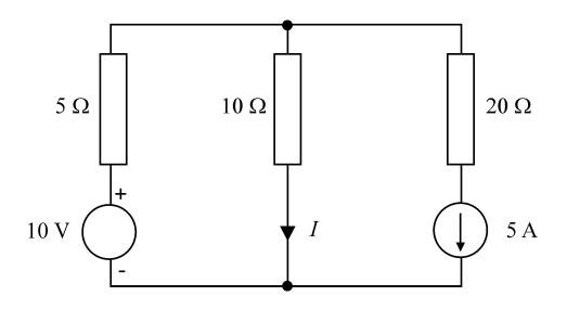
We could of course solve the problem directly by introducing a (clockwise) loop current I<sub>1</sub> into the left hand loop. The loop equation  $10=5I_1+10(I_1-5)$  yields  $I=I_1-5=-1$ Amp. We now confirm this result using the principle of superposition.
